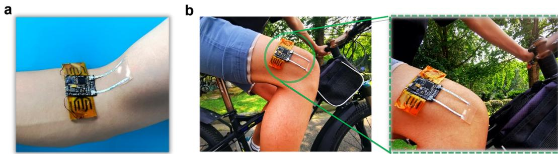
**Fig. S30.** The photographs of the wearable sensing system for human motion monitoring: (a) bicep curl and (b) bike riding.
