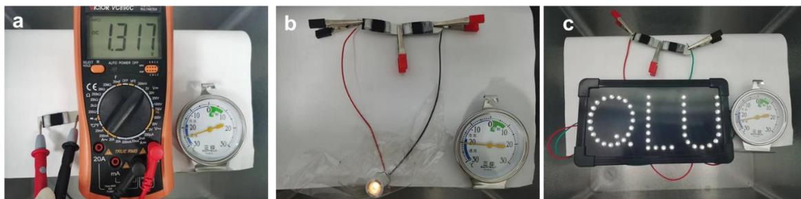
Fig. S48 (a) The potential of Wood-WTF-ZABs at low temperature; (b-c) an LEDs powered by two flexible Zn-air batteries at low temperature.
