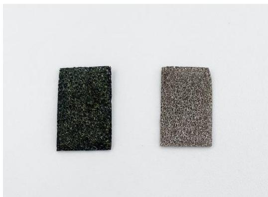
**Fig. S9.** Photograph of (a) PS<sub>480</sub>-*b*-P2VP<sub>490</sub> micellar film-decorated on nickel foam and (b) bare nickel foam after immersion in a solution of Ru<sup>3+</sup> ions in ethanol for 3 h.
