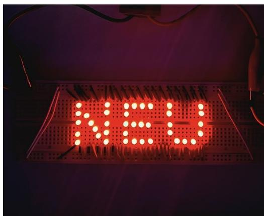
**Fig. S28** Digital image of the CFO-Zn || V<sub>2</sub>O<sub>5</sub>-NH<sub>4</sub><sup>+</sup> cell glowing the LED lights.
