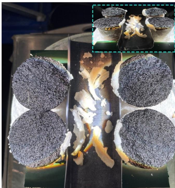
**Fig. S23.** An indoor scaled-up evaporation device constructed by 4 AEEs.
