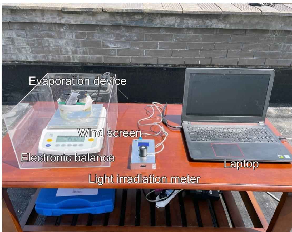
**Fig. S24.** Outdoor evaporation test system.
