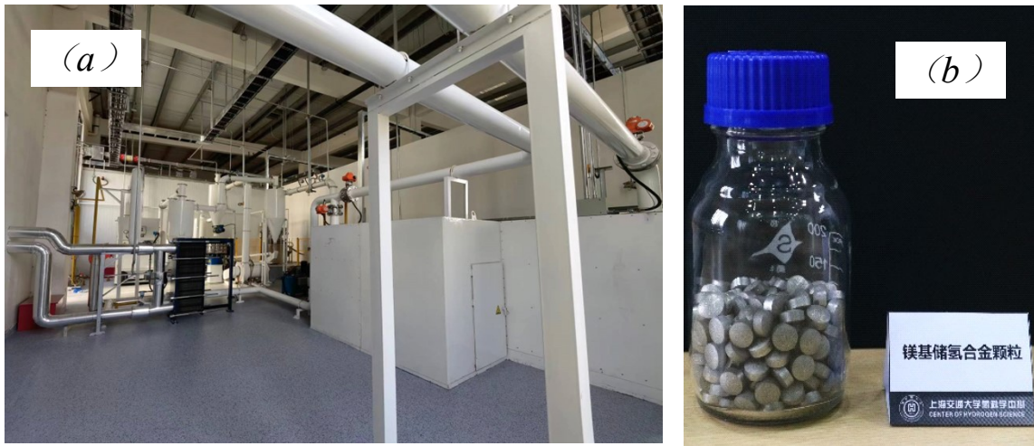
Figure S4. a Production line for magnesium-based solid-state hydrogen storage with an annual capacity of 100 tons; b Magnesium-based solid-state hydrogen storage pellets.
