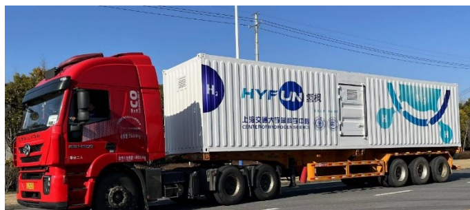
Figure S3. The world's leading ton-scale Mg-based solid-state hydrogen storage and transportation trailer.
