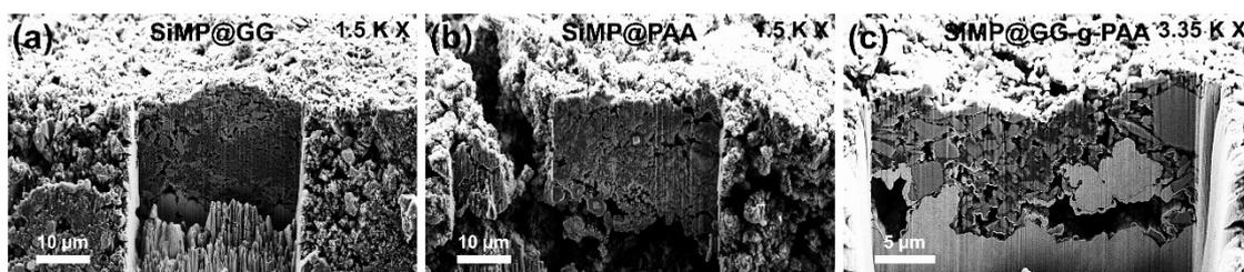
**Fig. S45** (a–c) High-resolution cross-sectional SEM images after FIB etching of the (a) SiMP@GG, (b) SiMP@PAA, and (c) SiMP@GG-g-PAA electrodes after 50 cycles at 0.2 C.
