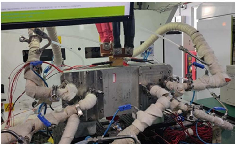
Fig. S4 Experimental setup for segmented fuel cell testing.
