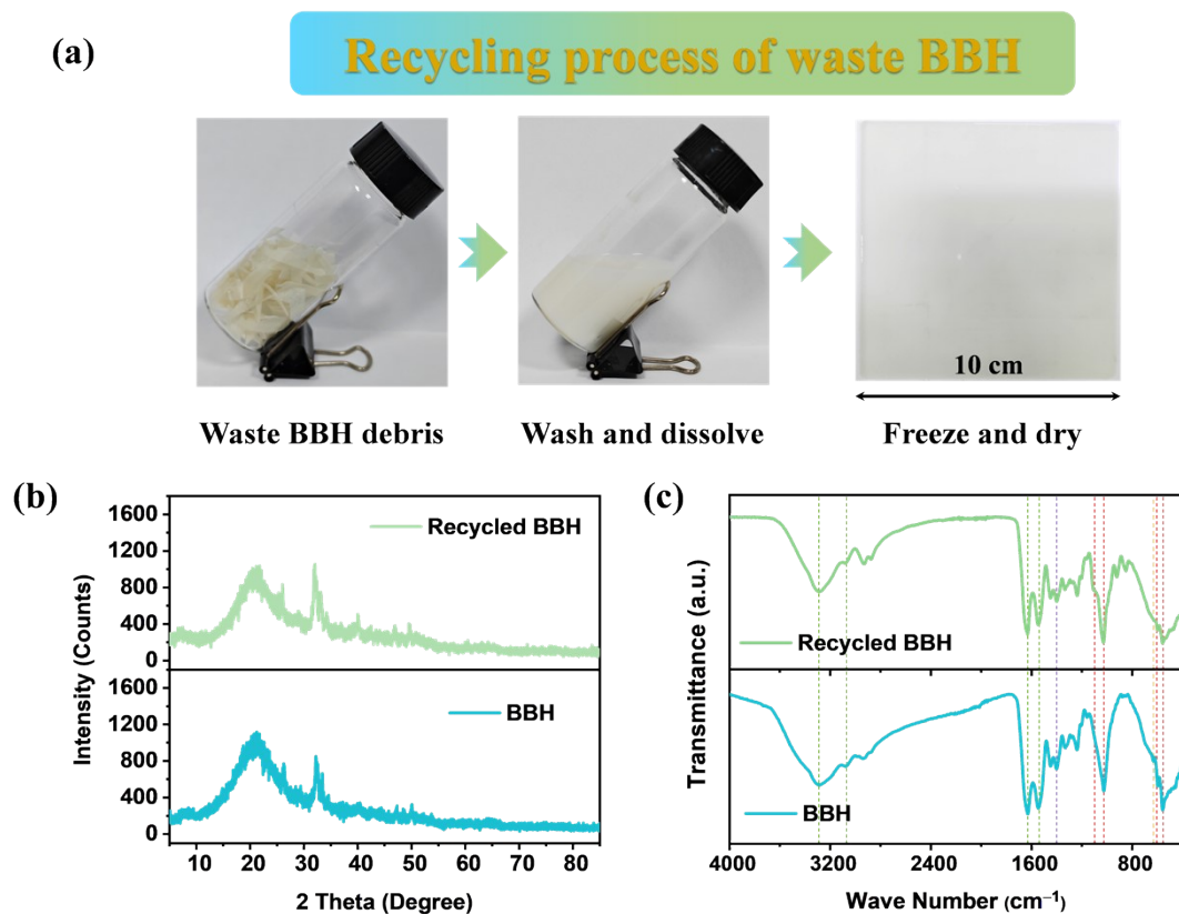
Figure S29. The recycling process and characterizations of Recycled BBH. (a) Recycling process of waste BBH. (b) XRD spectra of original BBH and Recycled BBH. (c) ATR-FTIR spectra of original BBH and Recycled BBH.
