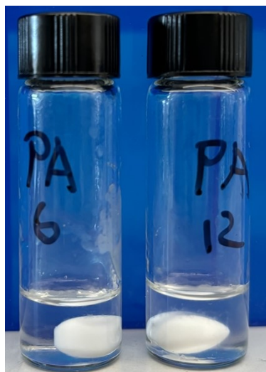
Fig. S3 The dissolution status of 2 wt.% PA 6 and PA 12 in 1M LiPF 6 in DEC.
