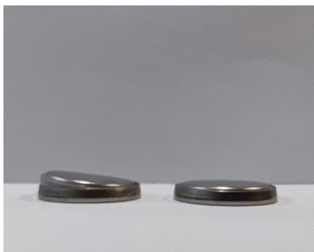
Figure S16. The state of the button cells after cycles in ZnSO 4 (left) and ZnSO 4 + BHED (right) electrolytes.
