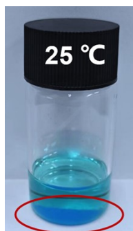
Fig. S7. The optical photograph of 0.5 m \text{CuSO}_4 in DMSO (DMSO with a molar fraction of 0.3).
