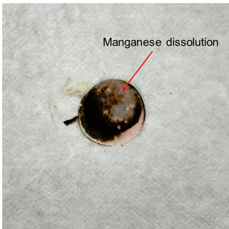
**Figure S35.** The photo of the separator that was retrieved from the Co-MnO<sub>2</sub> battery in 1 M CoCl<sub>2</sub> after cycling.
