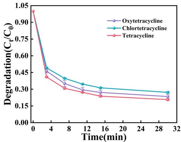
**Figure S3.** CNT catalyzed degradation of CTC, OTC, and TC *via* CaSO<sub>3</sub> activation. Reaction
