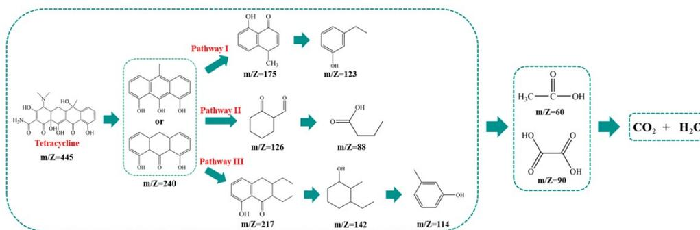
Figure S6. The possible TC degradation pathways over CNTs/CaSO<sub>3</sub> system.
