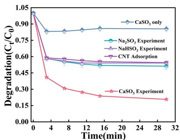
**Figure S2.** TC adsorption by only CNT, degradation by only CaSO<sub>3</sub> and comparison of TC degradation catalyzed by CNT with CaSO<sub>3</sub>, Na<sub>2</sub>SO<sub>3</sub> and NaHSO<sub>3</sub>. respectively. Reaction Conditions: 0.2 g/L of CNTs, 0.05 g/L of sulfites and 20 mg/L of TC at 30 °C.
