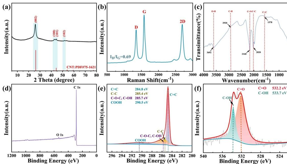
**Figure S1.** (a) XRD, (b) Raman spectra, (c) FT-IR, (d) Sum, (e) C 1s and (f) O 1s XPS of CNTs.
