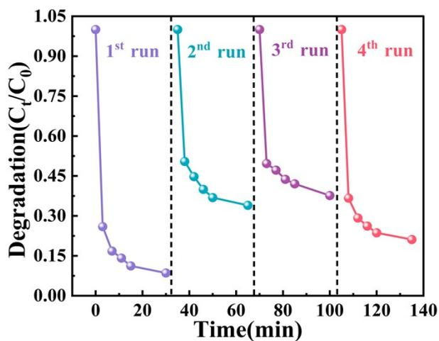
**Figure S4.** Stability of CNT in TC degradation. Reaction Conditions: 0.3 g/L of CNTs, 0.05 g/L
