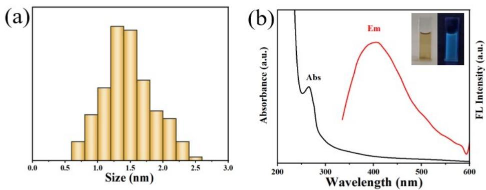
**Figure. S1** (a) Particle size distribution of TACDs, (b) Absorption and fluorescence emission spectra of TACDs.
