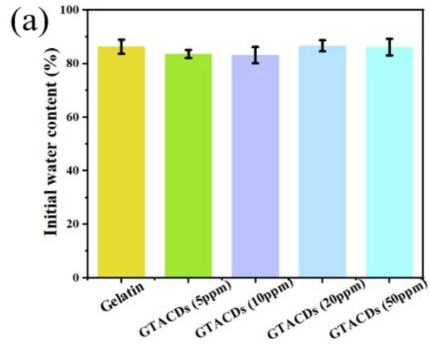
**Figure. S3** The initial water content (%) of Gelatin, GTACDs hydrogels (5, 10, 20, 50 ppm) (n=3).
