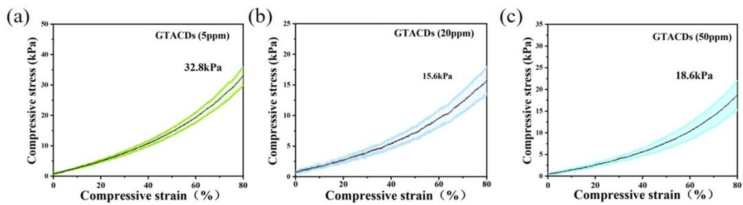
**Figure. S6** The compression-strain curves of GTACDs hydrogels (5, 20, 50 ppm) (n=3).
