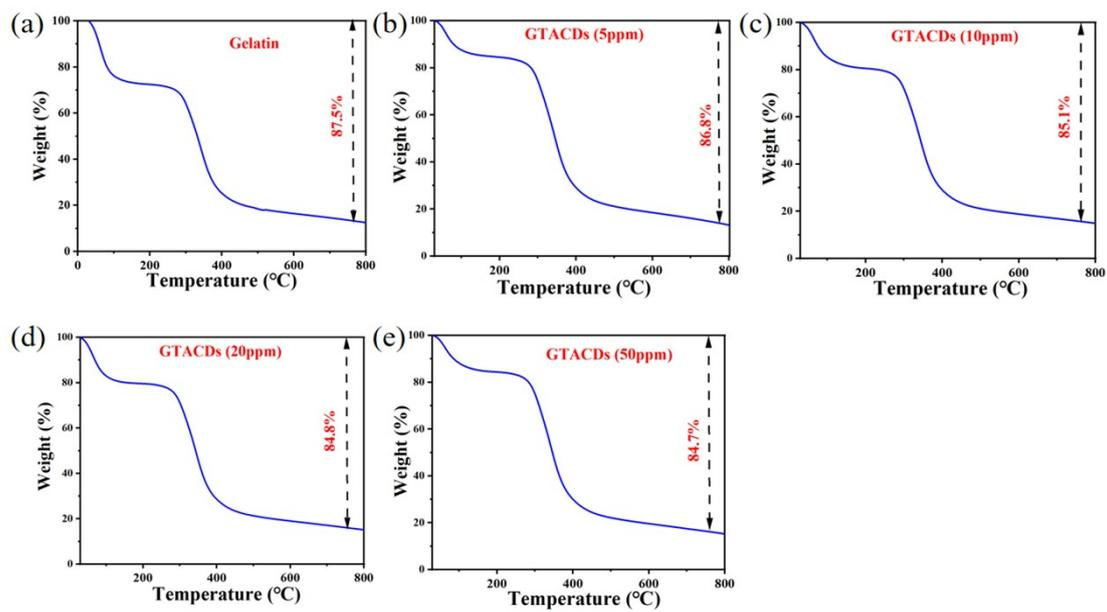
**Figure. S5** Thermal gravimetric analysis (TGA) curves of GTACDs hydrogels (5, 10, 20, 50 ppm).
