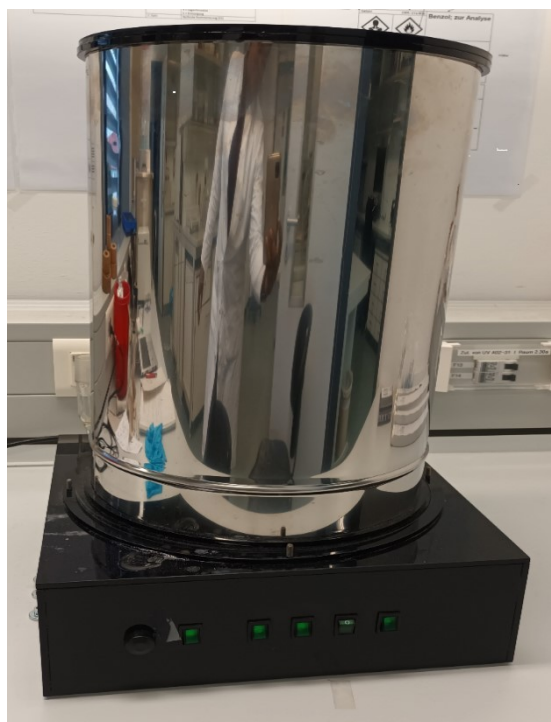
Figure S1. Homebuilt photoreactor: top image open and bottom image with the reflective jacket mounted.
