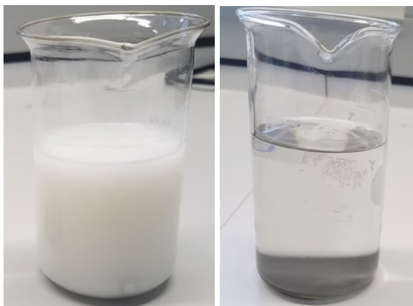
Figure S5. Comparison of 1 hour post-treatment recovery of pure titania (left) and titania hybrid clay nanocomposites (right) 6 These data clearly demonstrate that the composites are much easier to recover than pure titania particles. The latter do not sediment and are hard to separate from the liquid phase even via centrifugation.
