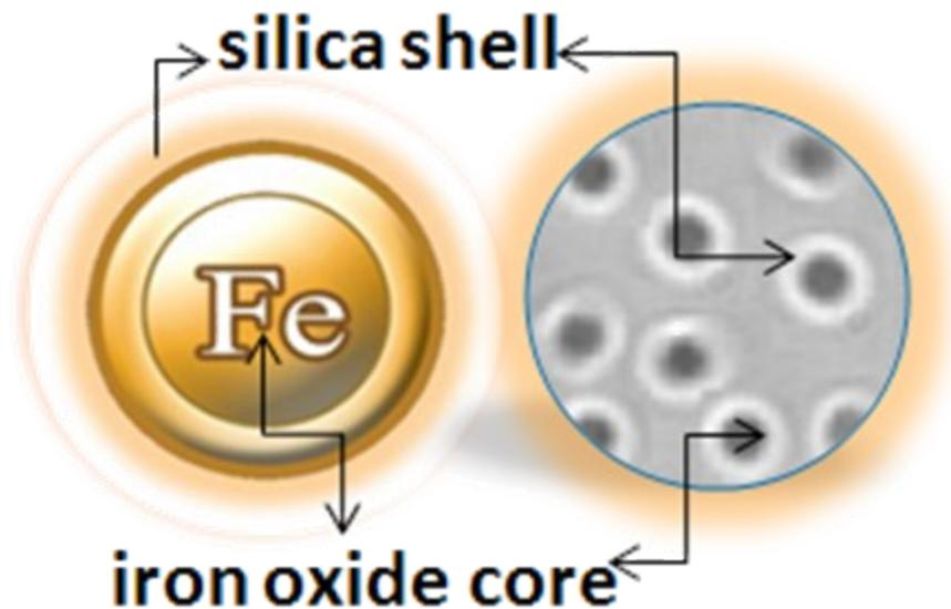
**Figure S1.** Transmission electron microscopy image of BcMag<sup>TM</sup> NHS-activated magnetic IOPs (image shared by the material supplier, Bioclone Inc., USA). The TEM image depicts the silica shell surrounding the iron oxide particles.
