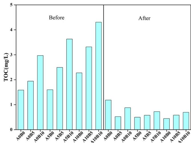
Figure S6 Changes in DOC during the chlorination process of BSA/SA samples with different concentration gradients. Reaction conditions: [initial chlorine concentration]<sub>0</sub> = 10 ± 0.2 mg/L, reaction time = 48 h, T = 25 ± 2 °C.
