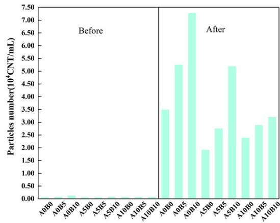
Figure S2 Changes in Particles number during the chlorination process of BSA/SA samples with different concentration gradients. Reaction conditions: [initial chlorine concentration]<sub>0</sub> = 10 ± 0.2 mg/L, reaction time = 48 h, T = 25 ± 2 °C.
