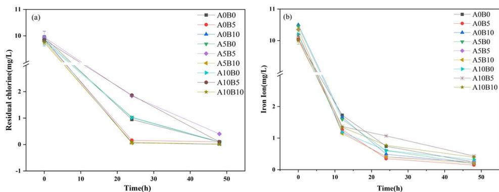
Figure S1 Changes in (a)residual chlorine and (b)iron concentrations during the chlorination process of BSA/SA samples with different concentration gradients. Reaction conditions: [initial chlorine concentration]<sub>0</sub> = 10 ± 0.2 mg/L, reaction time = 48 h, T = 25 ± 2 °C.
