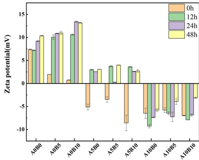
Figure S3 Changes in zeta potential during the chlorination process of BSA/SA samples with different concentration gradients. Reaction conditions: [initial chlorine concentration]<sub>0</sub> = 10 ± 0.2 mg/L, reaction time = 48 h, T = 25 ± 2 °C.
