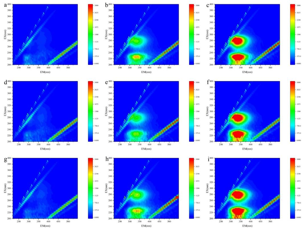
Figure S4 3D-EEM contour plots of BSA/SA samples with different concentration gradients before chlorination reaction. Reaction conditions: [initial chlorine concentration]<sub>0</sub> = 10 ± 0.2 mg/L, reaction time = 48 h, T = 25 ± 2 °C.
