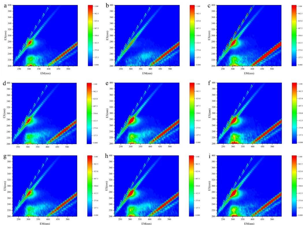
Figure S5 3D-EEM contour plots of BSA/SA samples with different concentration gradients after chlorination reaction. Reaction conditions: [initial chlorine concentration]<sub>0</sub> = 10 ± 0.2 mg/L, reaction time = 48 h, T = 25 ± 2 °C.
