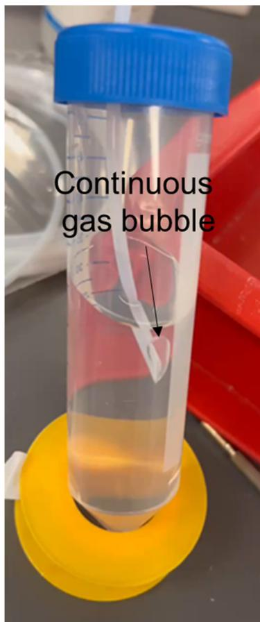
**Fig. S6.** Picture taken at the outlet of the reversed GDE cell under a current density of 80 mA/cm<sup>2</sup>. Continuous output of gas can be observed throughout (Supplementary Video 1).
