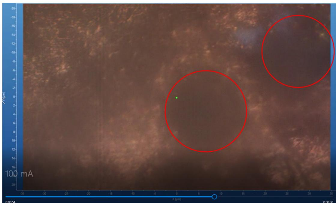
**Fig. S11.** Screenshot of the gas growth at a current density of  $100 \text{ mA/cm}^2$ . We could see two adjacent bubbles, which had been pointed by the red cycles.
