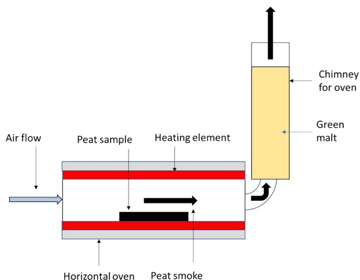
**Figure S3.** Diagram of the SWRI laboratory scale peating apparatus.
