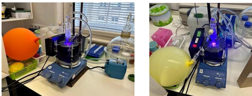
**Figure S17.** Experimental setup for the preparative photocatalytic oxidation of benzylic alcohols with oxygen balloon under LED irradiation (400 nm) and with water cooling system.
