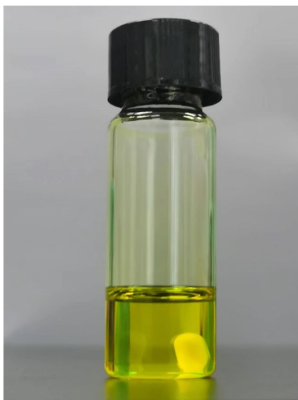
Fig. S1 The optical image solution of FA-based quasi-2D perovskite in TEP.
