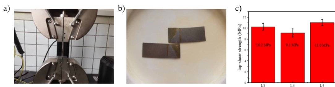
Figure S7 Adhesive test results. a) equipment for lap-shear test; b) a photo of failed Q235 steel plates bonded using L5 glue. Clear adhesive failure can be observed; c) lap-shear strength of ELO-based vitrimers.
