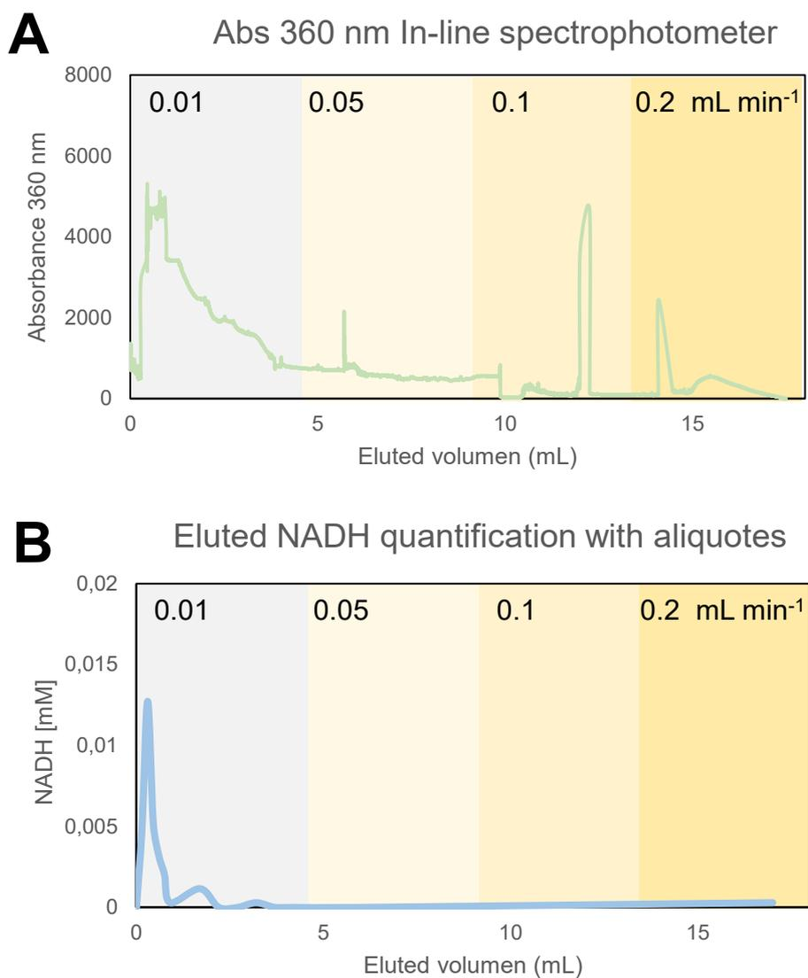
**Figure S8. Eluted NADH during continuous flow optimisation 200 mM 1a reduction at different flow rates with TtHBDH ssHB**
