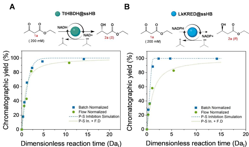
**Figure S9. Comparison of simulated (dashed line) and real (square/circle) data of 1a conversion**
