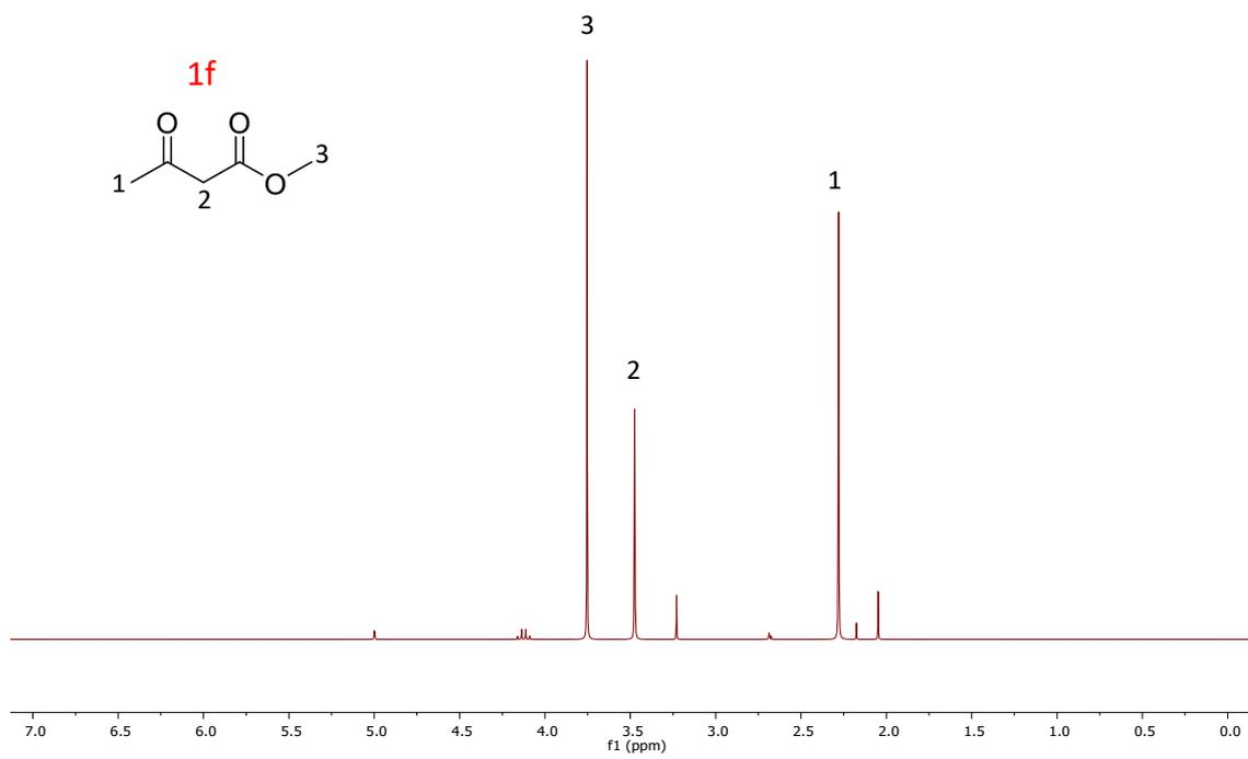
**Figure S15. <sup>1</sup>H NMR of 1f (300 MHz, Chloroform, 298 K)**
