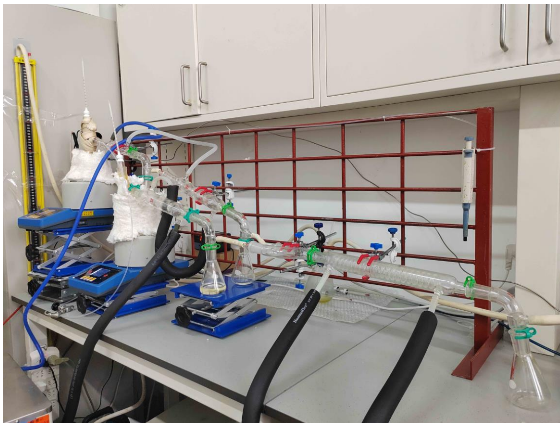
Fig. S18 Physical diagram of the two-stage reaction of FDC and THFDC decomposition.
