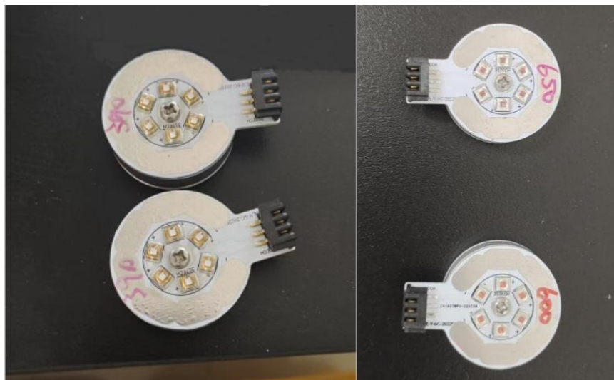
Figure S7. Independent removable replacement light source
