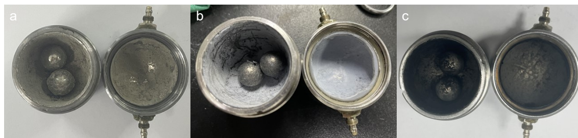
Figure S5. The status of the reaction mixtures after ball milling using different amounts of \alpha -CD (a 2.0 equiv. \alpha -CD, b 0.4 equiv. \alpha -CD, c 0.1 equiv. \alpha -CD)
