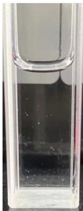
Figure S9. Tests on Tyndall effect: HBr and BnOH in acetone solution
