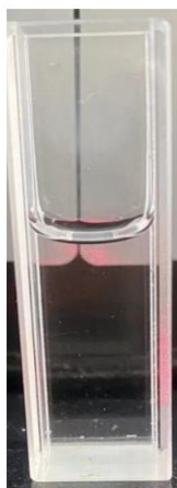
Figure S10. Tests on Tyndall effect: H 2 O and BnOH in EtOAc solution
