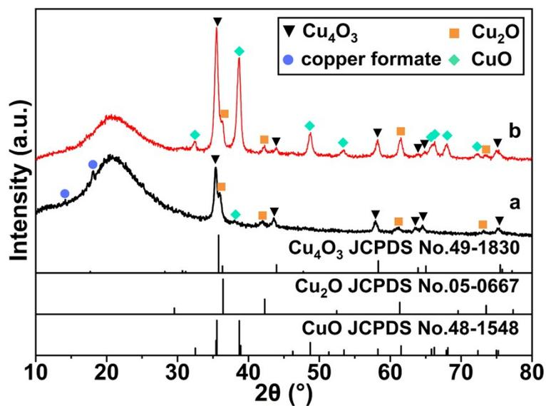
**Figure S3.** XRD spectra of the sintered product of copper formate/CSBC precursor after the solid-state sintering process at different sintering temperature. (a) sintering at 220 °C for 12 min; (b) sintering at 240 °C for 12 min.
