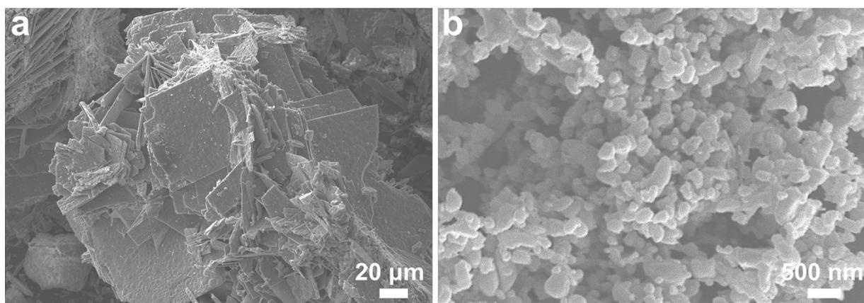
**Figure S1.** SEM images of copper formate. (a) untreated sample, (b) after the BM-1 process.
