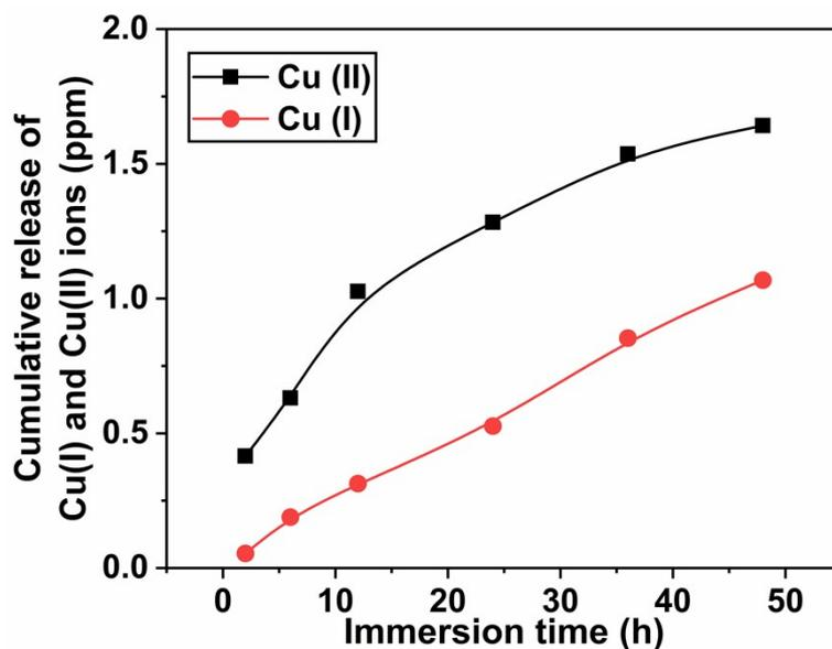
**Figure S7.** Cumulative release of Cu(I) and Cu(II) ions for the  $\text{Cu}_4\text{O}_3/\text{CSBC}$  composite during the 48-hour immersion experiment. The data were obtained as follows,
