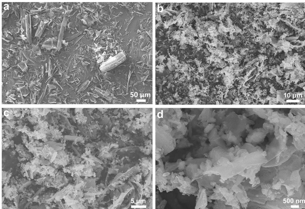
**Figure S2.** SEM images of (a) CSBC and (b-d) the copper formate/CSBC precursor.
