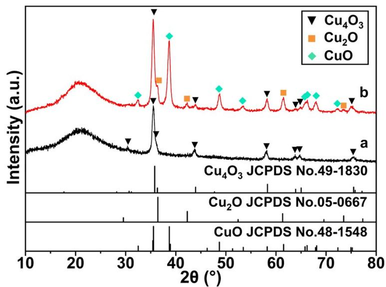
**Figure S4.** XRD spectra of the sintered products for the CSBC supporting capacity experiments on  $\text{Cu}_4\text{O}_3$ . (a) support amount of 10 wt.% for  $\text{Cu}_4\text{O}_3$ ; (b) support amount of 20 wt.% for  $\text{Cu}_4\text{O}_3$ .
