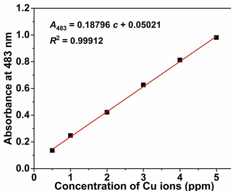
**Figure S6.** Standard curve between the absorbance of BCS at 483 nm and the concentrations of Cu ions. The linear regression equation was obtained from the standard curve as follows,
