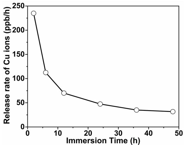
**Figure S5.** Release rate of Cu ions for the  $\text{Cu}_4\text{O}_3/\text{CSBC}$  composite during the 48-hour immersion experiment. The data were analyzed based on the differences in the cumulative release of Cu ions during each test period.
