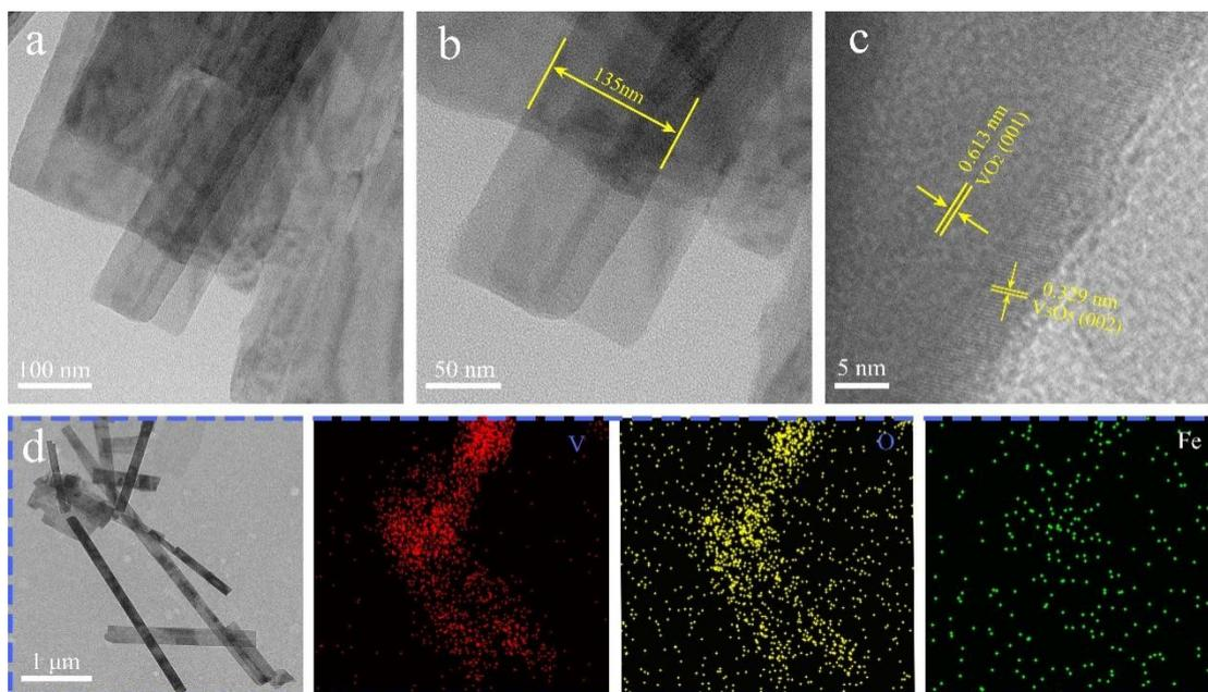
Fig. S5 (a), (b) TEM and (c) HRTEM images of  $\text{VO}_2(\text{B})/\text{V}_3\text{O}_5$ . (d) Element mapping of V, Fe, O in  $\text{VO}_2(\text{B})/\text{V}_3\text{O}_5$
