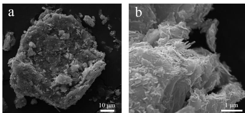
Fig. S4 SEM images of Fe<sub>0.1</sub>VO<sub>2</sub>(B)/V<sub>3</sub>O<sub>5</sub> with no addition of PEG-4000
