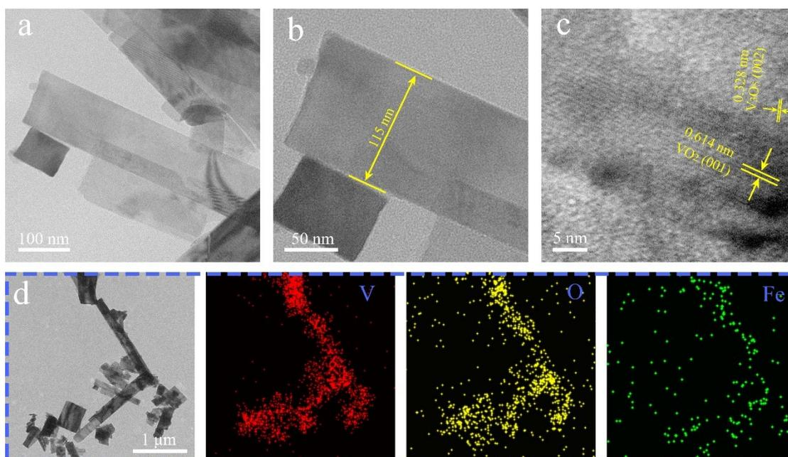
Fig. S6 (a), (b) TEM and (c) HRTEM images of  $\text{Fe}_{0.05}\text{VO}_2(\text{B})/\text{V}_3\text{O}_5$ . (d) Element mapping of V, Fe, O in  $\text{Fe}_{0.05}\text{VO}_2(\text{B})/\text{V}_3\text{O}_5$
