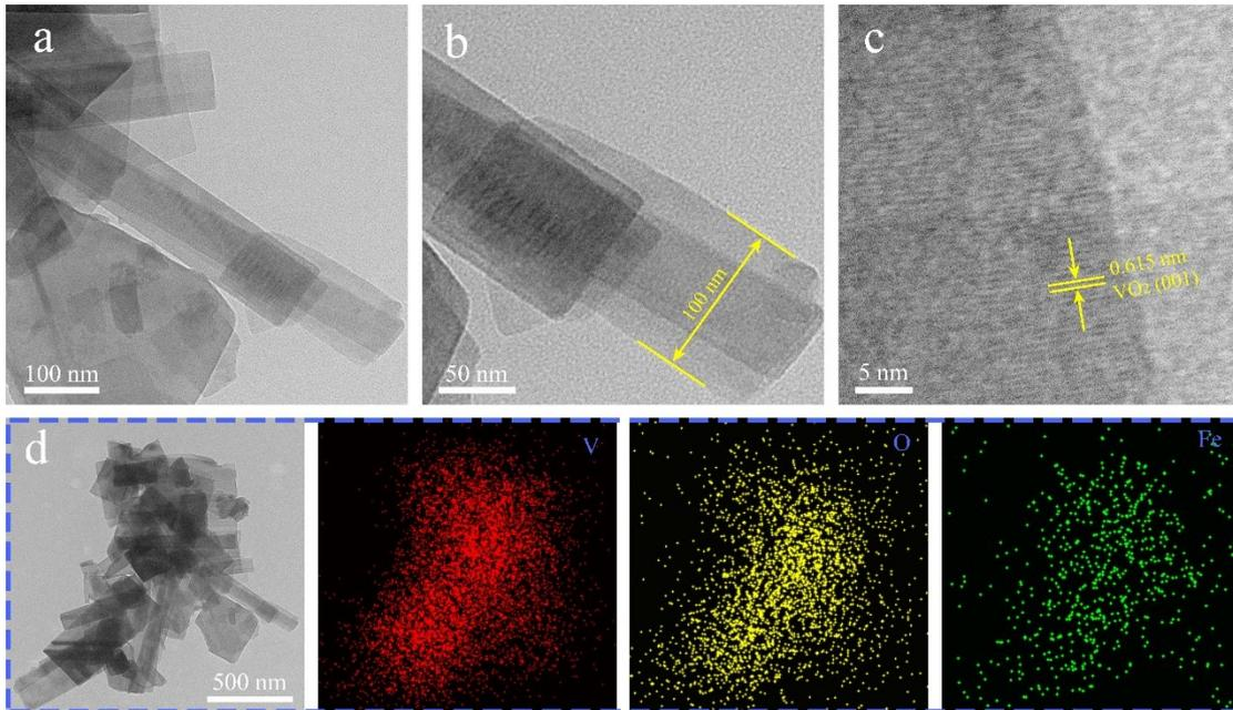
Fig. S7 (a), (b) TEM and (c) HRTEM images of  $\text{Fe}_{0.15}\text{VO}_2(\text{B})/\text{V}_3\text{O}_5$ . (d) Element mapping of V, Fe, O in  $\text{Fe}_{0.15}\text{VO}_2(\text{B})/\text{V}_3\text{O}_5$
