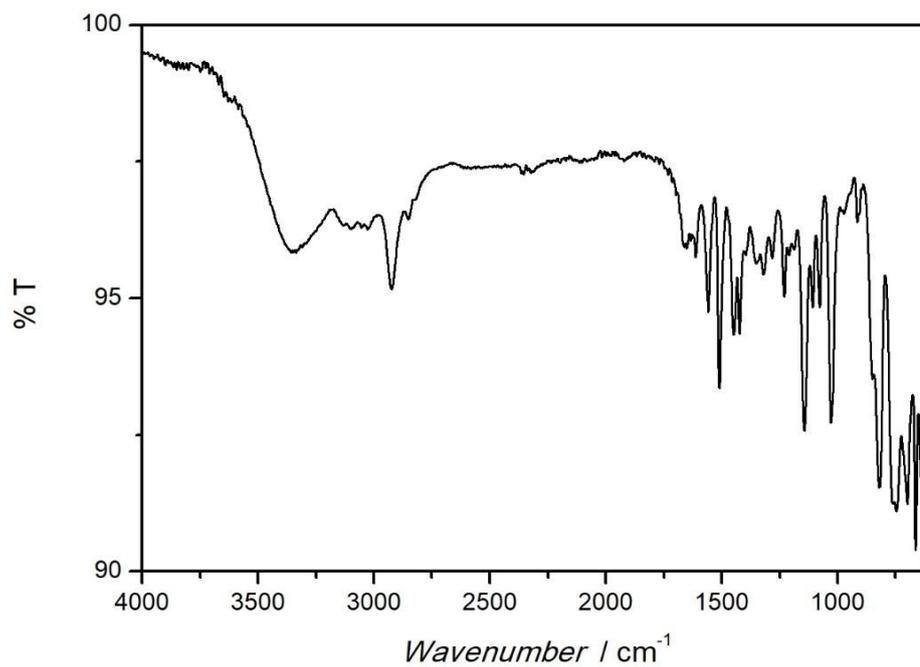
**Fig. S7** FT-ATR-IR spectra of imidazole polymer 2.
