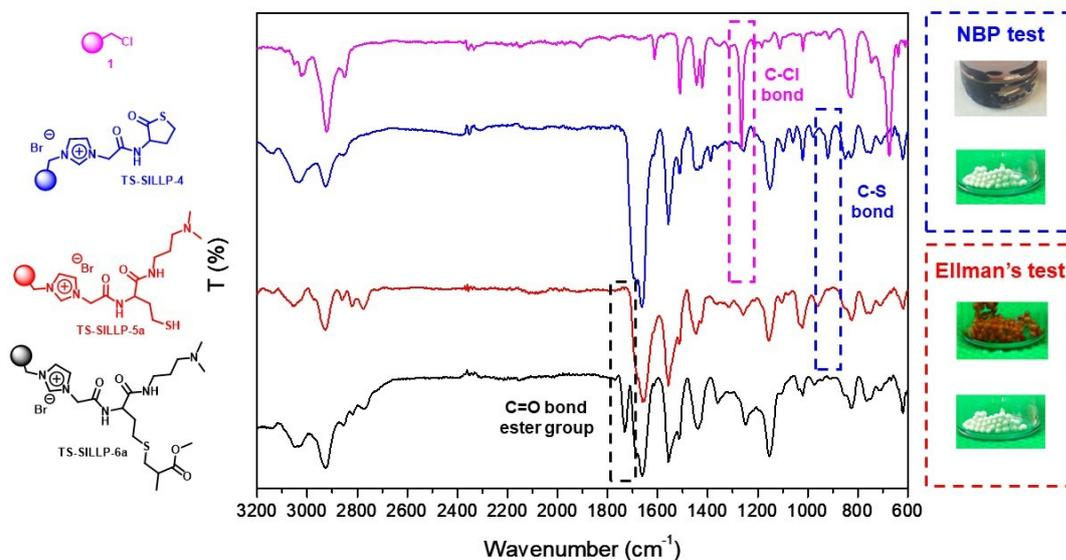
**Fig. S1** FT-IR spectra for the synthesis monitoring of Solid-Phased task-specific supported ILs library. NBP test to check the successful modification of Merrifield resin and Ellman's test to check the successful opening of the thiolactone rings.
