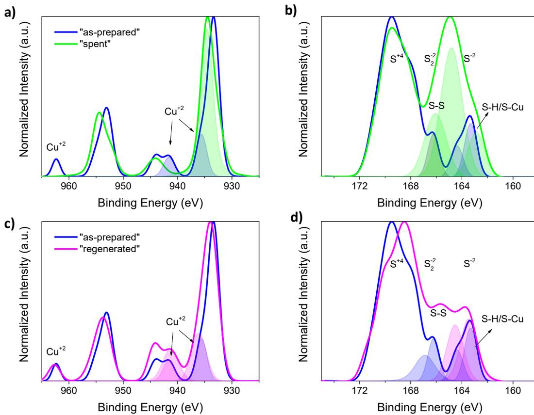
**Fig. S4** a) Cu 2p (a) and b) S 2p regions of the XPS for the **Cu(OAc)<sub>2</sub>-TS-SILLP-5a** "as prepared" (blue) and "spent" (green). c) Cu 2p and d) S 2p regions of the XPS for the **RB-Cu(OAc)<sub>2</sub>-TS-SILLP-5a** "as prepared" (blue) and "regenerated" after 14<sup>th</sup> regeneration cycles (magenta).
