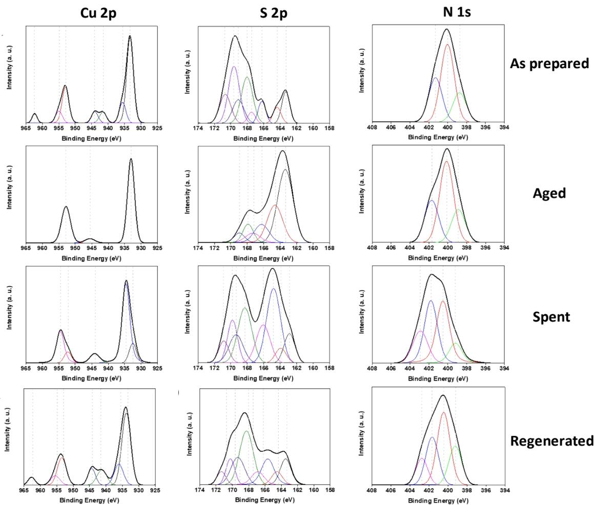
**Fig. S5** XPS of the Cu 2p (left), S 2p (middle) and N1s (right) for the as prepared (1<sup>st</sup> line), aged (2<sup>nd</sup> line), spent (3<sup>th</sup> line) and regenerated Cu(OAc)<sub>2</sub>-TS-SILLP-5a (4<sup>th</sup> line).
