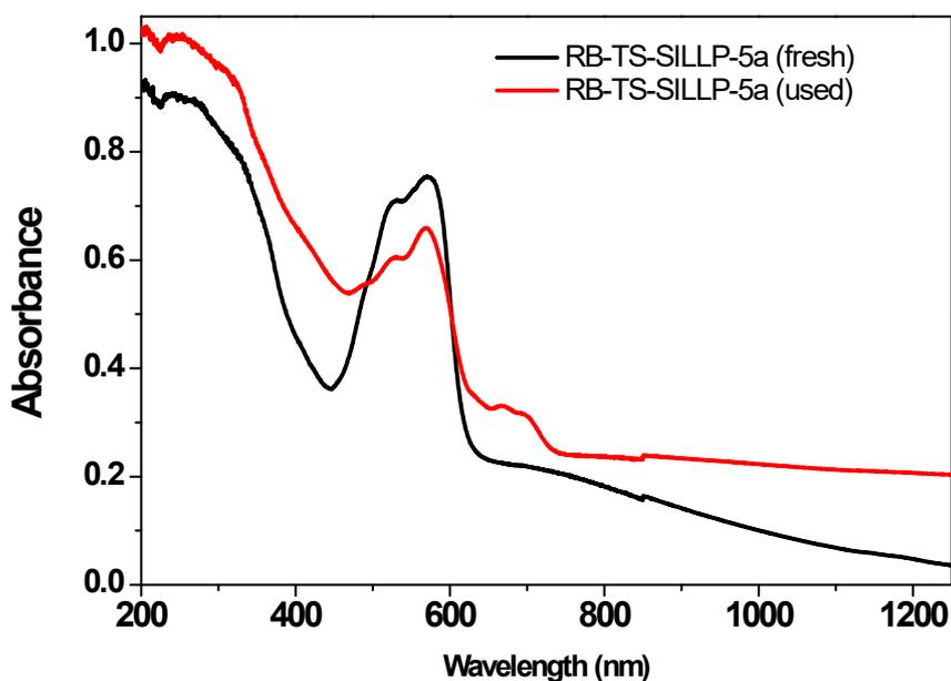
**Fig. S6** UV spectra of **RB-Cu(OAc)<sub>2</sub>-TS-SILLP-5a** before (fresh) and after (used after 15<sup>th</sup> reaction cycles 14<sup>th</sup> regeneration cycles) for the reaction between **7a** and **8a**.
