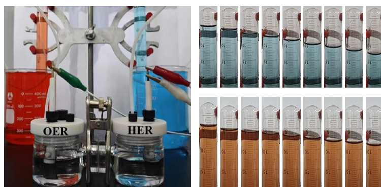
Figure S20 The device for monitoring the rates of H 2 and O 2 production.
