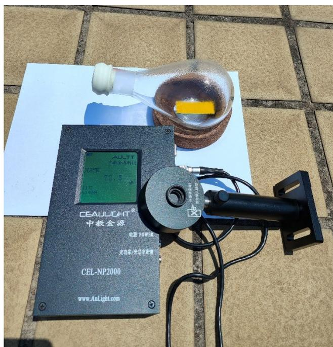
**Figure S16.** The gas-phase CO<sub>2</sub> photoreduction experiment over TPT-BBT at East China University of Technology (Nanchang campus, China) on Aug 6<sup>th</sup>, 2024. Reaction time: from 13:00 pm to 16:00 pm, solar intensity:  $\sim 72.5 \text{ mW/cm}^2$ , outdoor temperature: 41 °C at 13:00 pm.
