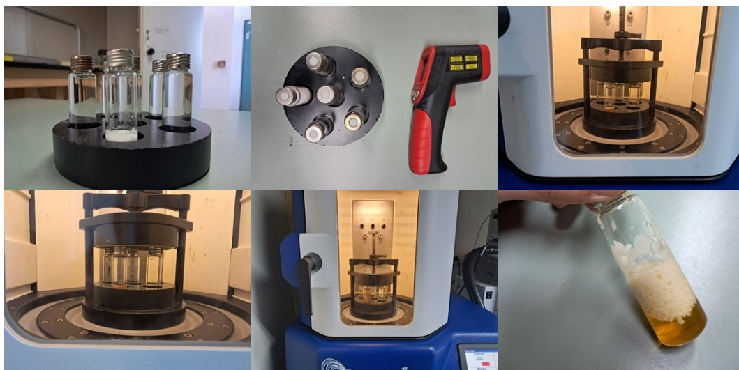
Figure 5. Loading and running of the gram-scale on the LAB RAM II along with the Infrared thermometer used for checking the temperature during the reaction.
