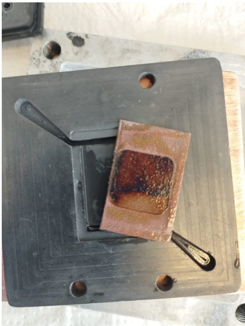
Fig. S16 Spent GDE with graphite holding plate, water droplets have permeated through the GDE.
