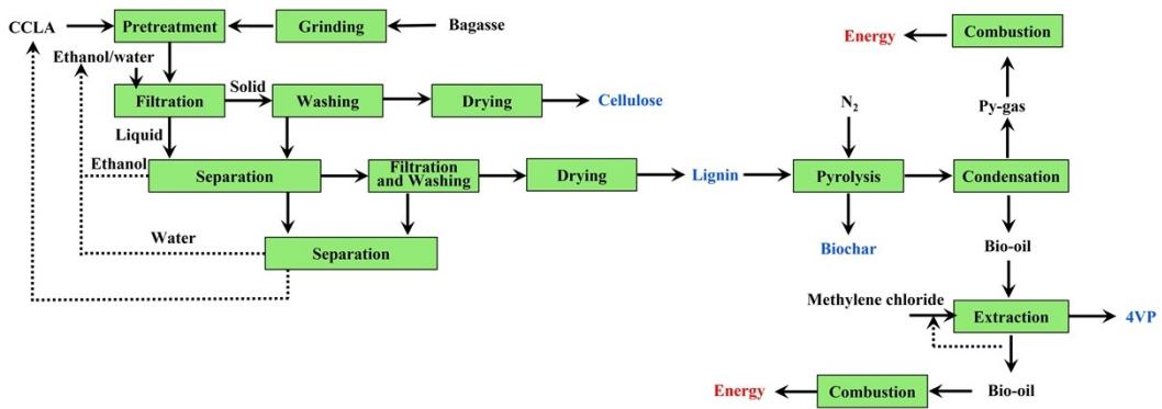
Fig S4. The block diagram of the TEA model for 4VP production
