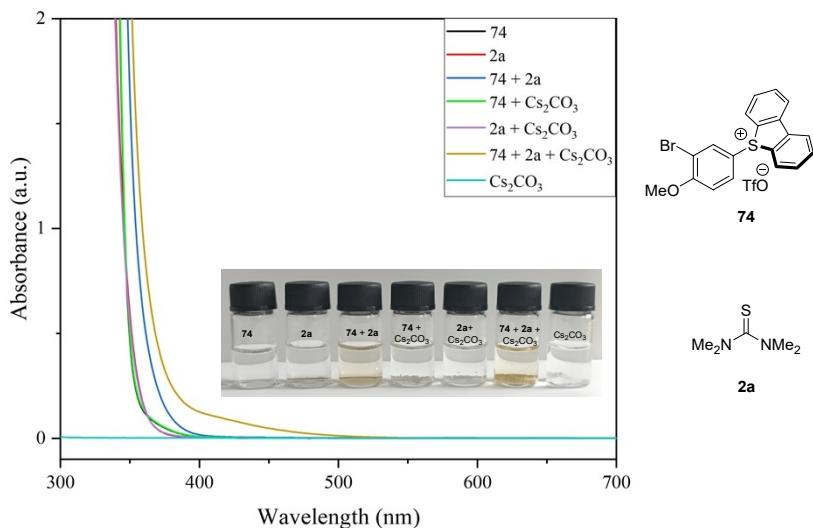
**Figure S7.** The absorption spectra in solution were recorded on a UNIC 4802 UV/VIS double beam spectrophotometer in a 1.0 cm length quartz cell. All compounds were dissolved in  $\text{CH}_3\text{CN}$  and measured at  $25^\circ\text{C}$ .  $[74] = 0.3 \text{ M}$ ,  $[2\text{a}] = 0.6 \text{ M}$ ,  $[\text{Cs}_2\text{CO}_3] = 0.4 \text{ M}$ .
