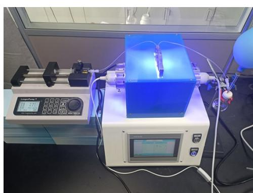
**Figure S2.** Flow set-up with light irradiation
