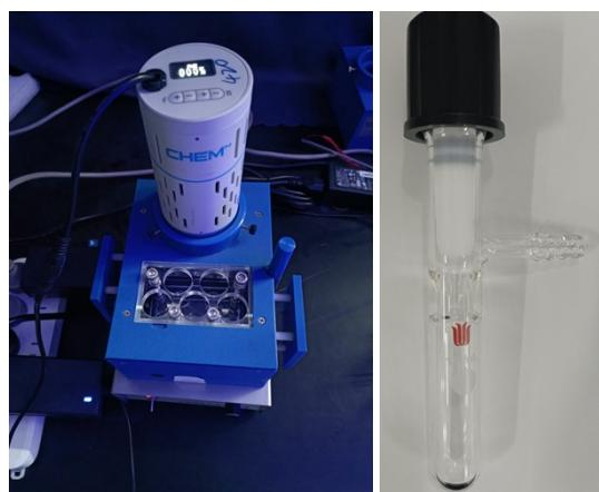
**Figure S1.** Photo-reaction setup and reaction tube
