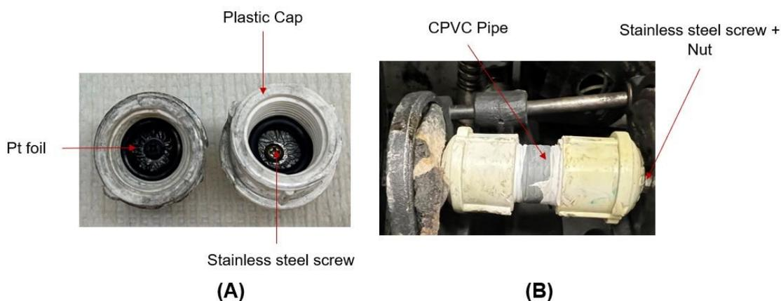
**Figure S7.** A) Parts of modified MEC-7 (Top view), B) Assembled modified MEC-7.
