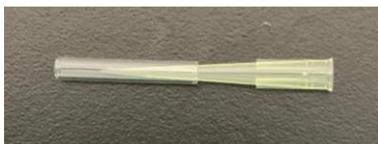
3. **Curing:** The coated glass inserts were mounted on a hand-made wire stand and incubated at 60 °C for 1 h. This coating process was repeated once, followed by overnight incubation at 60 °C to ensure complete curing.
