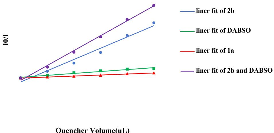
**Figure S6.** Stern-Volmer analysis for 4CzIPN with **1a**, **2b** and DABSO
