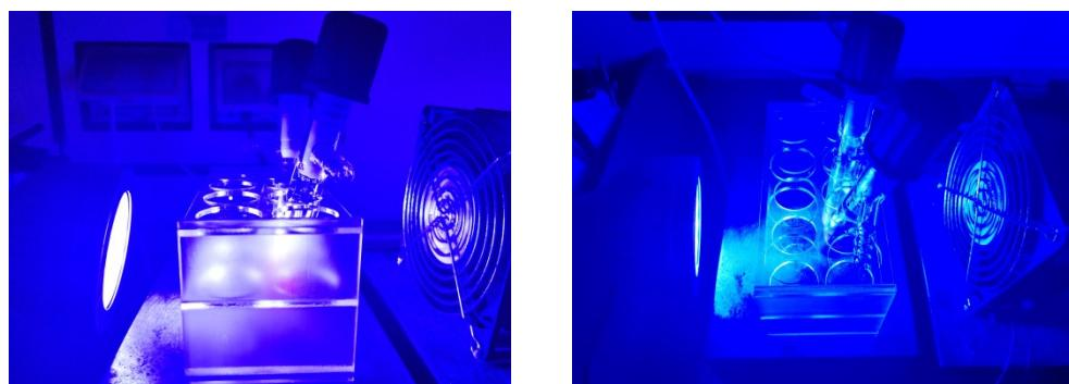
**Figure S1** Photograph of the Reaction Setup (Blue LED, 450-460 nm)
