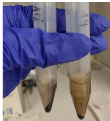
Figure S2. Pictures of the \text{Co}_3\text{O}_4^{\text{heptOH}} and KuQ3P suspension before mixing ( left ) and of the centrifuged suspension after stirring KuQ3P together with \text{Co}_3\text{O}_4^{\text{heptOH}} NPs ( right ).
