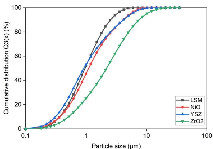
**Fig. S1** Cumulative volume (mass) weighted particle size distributions obtained by laser diffraction with dry high intensity dispersing
