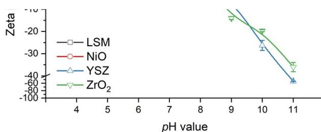
**Fig. S3** Effect of pH on the zeta potentials of the HTL materials. Surface charge of the electrode materials (LSM and NiO) remains positive with increase in the pH. The lines are guides for the eye. The error bars indicate 95% confidence intervals.
