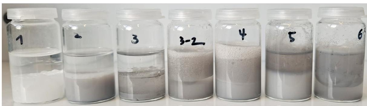
**Fig. S5** Effect of different combinations of surfactant and dispersant at different pH. From left to right 1 to 6
