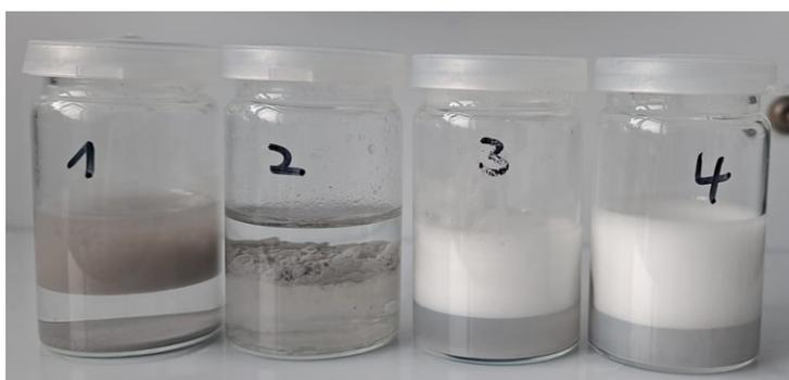
**Fig. S6** Particle mixtures (NiO, YSZ, and  $ZrO_2$ ) with different combinations of surfactant, dispersant, ultrasonic treatment
