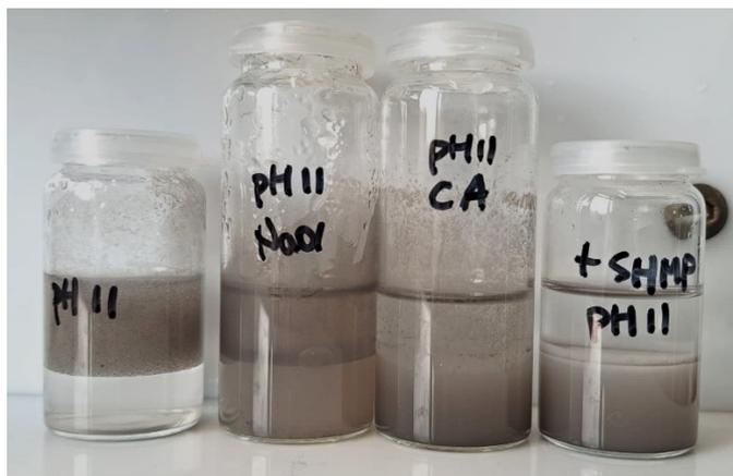
**Fig. S4** Effect of different types of dispersants in NiO dispersions at pH 11 From left to right: no dispersant (reference), sodium oleate (NaOl), citric acid (CA), and sodium hexametaphosphate (SHMP)
