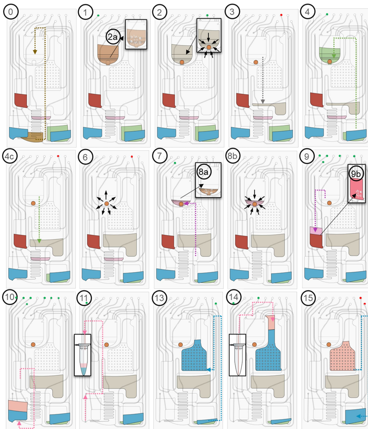
Fig. S13 Schematics illustrating the displacement of liquid on the cartridge during different stages of the process. Arrows indicate the direction of flow; activated ports are highlighted in green or red, representing the application of positive or negative pressure, respectively. A video recording of the actual sample-to-answer workflow using colored solutions is provided as a separate file to the ESI.
