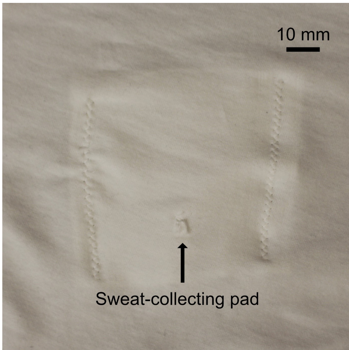
Figure S4: Photograph from inside the T-shirt with the sweat-indicating stitched microfluidic device attached to it on the outside (not visible), before use. Visible are the stitches with non-wicking nylon thread that connects the device to the T-shirt's fabric and the sweat-collecting pad made from a non-woven cotton pad that is the only part of the device on the inside of the T-shirt and touches the skin of the wearer, isolating the user from any reactants.
