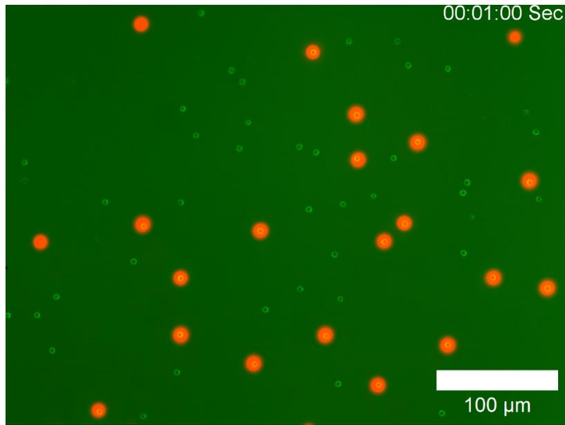
**Movie S1.** 10 μm red fluorescent polystyrene beads in water are trapped by 5 μm air cavities at the acoustic excitation of 3 MHz and 17 V<sub>pp</sub>.
