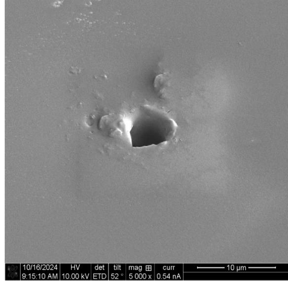
**Fig. S7:** SEM images of air cavities before and after laser-induced destruction. **(a)** Three intact air cavities with thin membranes, highlighted by red dashed circles. The average membrane diameter is approximately 2 μm. **(b)** An air cavity after exposure to a 1030 nm near-infrared laser, showing the membrane destroyed with an average hole diameter of around 4 μm.
