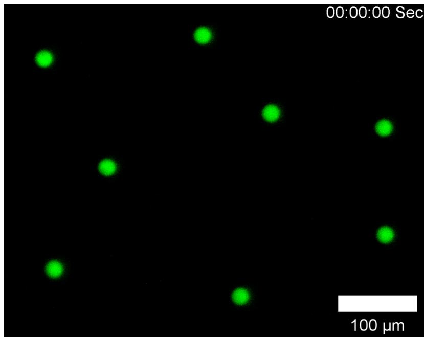
**Movie S4.** 10  $\mu\text{m}$  green fluorescent polystyrene microspheres initially trapped by 5  $\mu\text{m}$  air cavities at the acoustic excitation of 3 MHz and 17  $V_{pp}$ . Upon laser activation, the air cavities are selectively disrupted, releasing the microspheres one by one. The released particles are then flushed downstream by the background flow.
