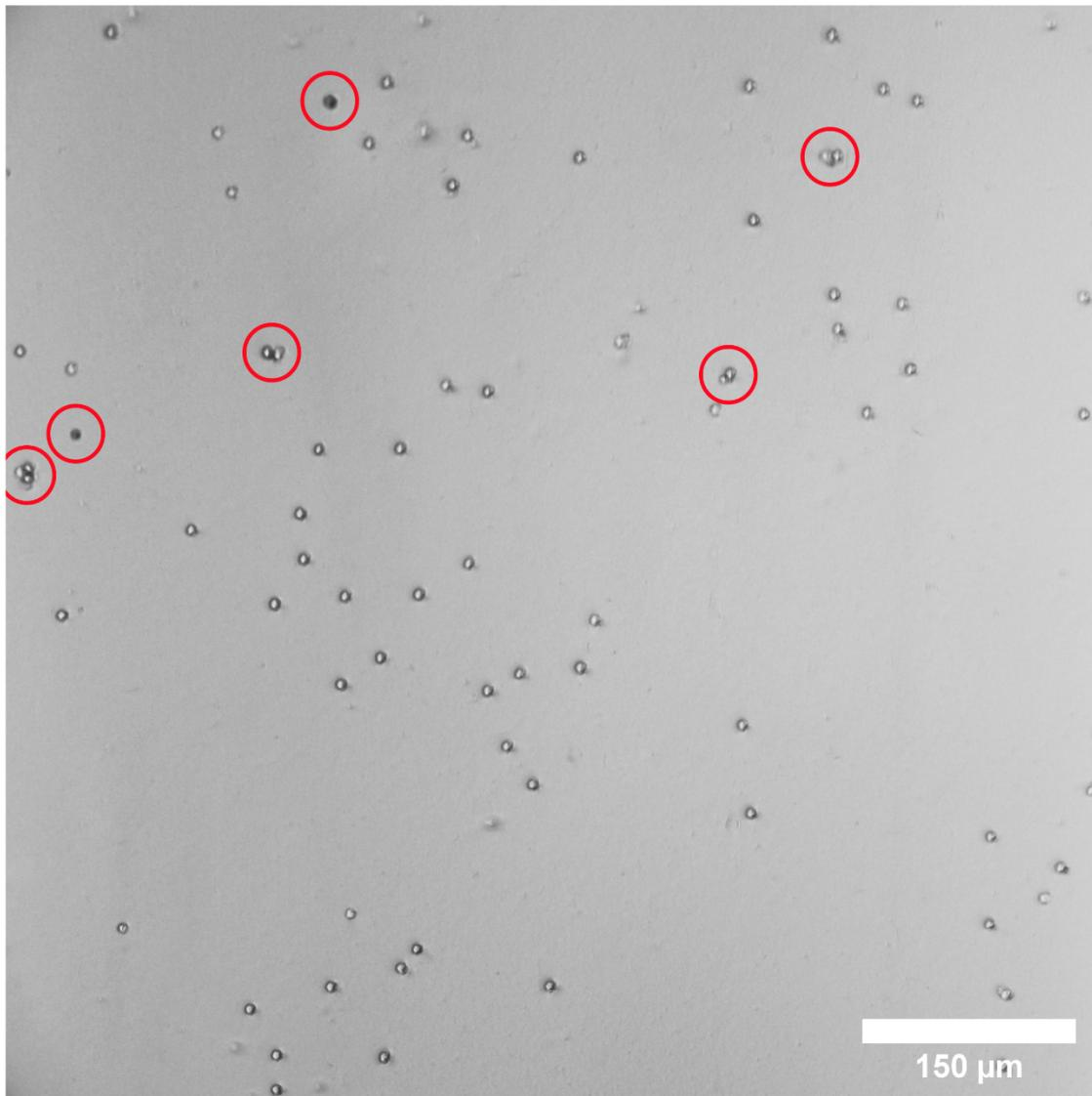
**Fig. S10:** Bright-field microscope image of air cavities on the device. Non-functional air cavities, such as those with defects (solid black circles) or cases where two cavities are stuck together, are highlighted with red circles. The functional air cavities account for approximately 90% of the total fabricated air cavities.
