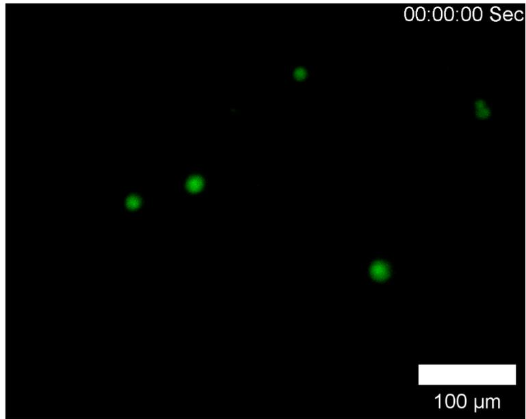
**Movie S5.** Green fluorescent A20 lymphoma cells are trapped in place by  $5\ \mu\text{m}$  air cavities at the acoustic excitation of 3 MHz and 17 Vpp. When the air cavities are selectively disrupted by the laser, the cells are released one by one and subsequently flushed downstream.
