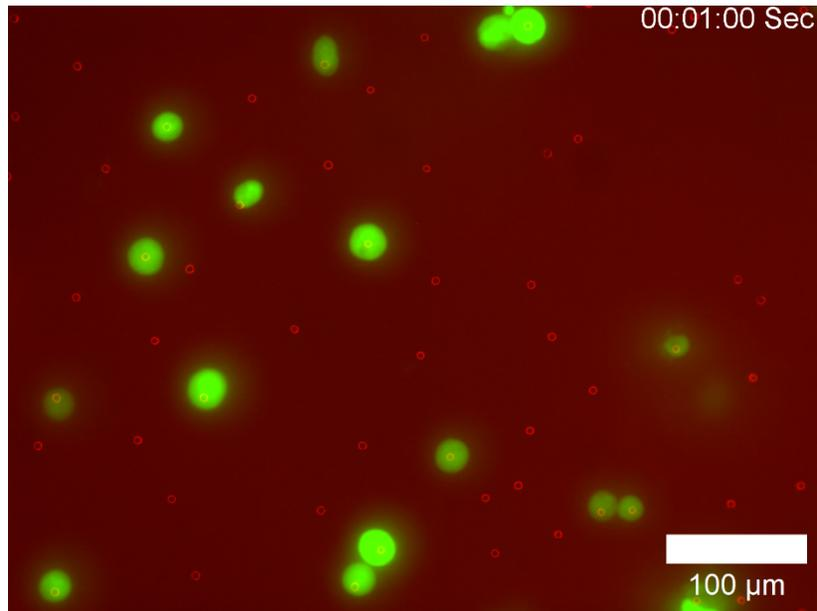
**Movie S3.** LNCap cells in culture medium are trapped by 5  $\mu\text{m}$  air cavities at the acoustic excitation of 3 MHz and 17  $V_{pp}$ . The size of the cells ranges from 20 to 30  $\mu\text{m}$ .
