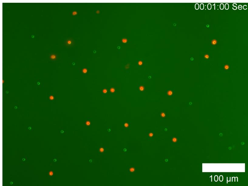
**Movie S2.** A20 lymphoma cells in culture medium are trapped by 5 μm air cavities at the acoustic excitation of 3 MHz and 17 V<sub>pp</sub>. The size of the cells ranges from 8 to 15 μm.
