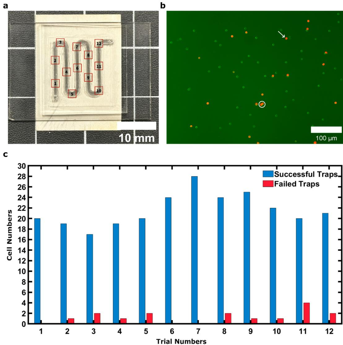
**Fig. 9S:** (a) The 12 examination areas sampled along the fluid channel. (b) An example image illustrating failed single-cell traps, either due to cell adhesion to the device surface or cell clustering. (c) A summary of the cell counts in the 12 examination areas. Of the 275 cells introduced into the observed regions, 259 single cells were successfully trapped, resulting in a single-cell trapping efficiency of 94.09% with a standard deviation of  $\pm 4.75\%$ .
