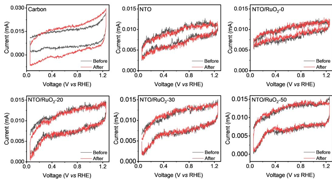
**Figure S7.** Cyclic voltammograms of carbon, NTO nanoparticles, and macroporous NTO/RuO<sub>2</sub> particles with varying RuO<sub>2</sub> binder contents before and after applying a potential of 1.3 V vs Ag/AgCl for 10 minutes.
