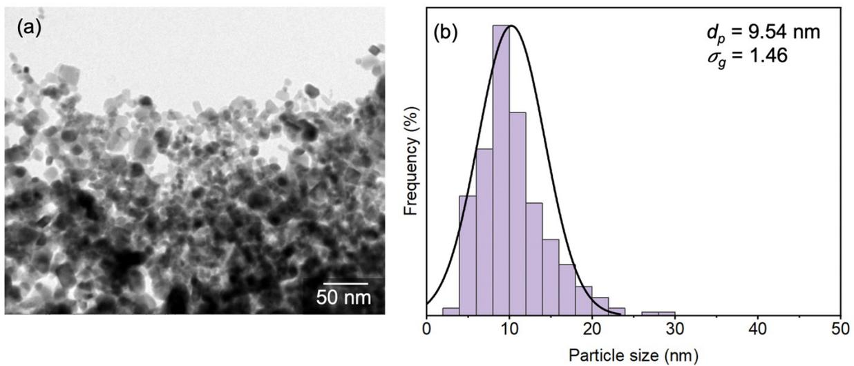
**Figure S6.** (a)TEM image and (b) size distribution chart of NTO nanoparticles.
