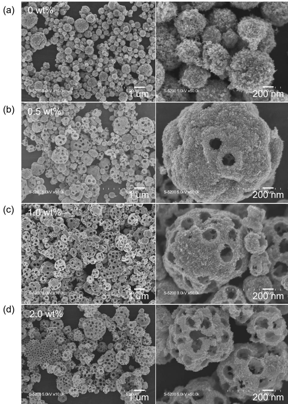
**Figure S1.** SEM images of macroporous NTO/RuO<sub>2</sub>-50 particles with different PMMA concentrations: (a) 0 wt.%, (b) 0.5 wt.%, (c) 1.0 wt.%, and (d) 2.0 wt.%.
