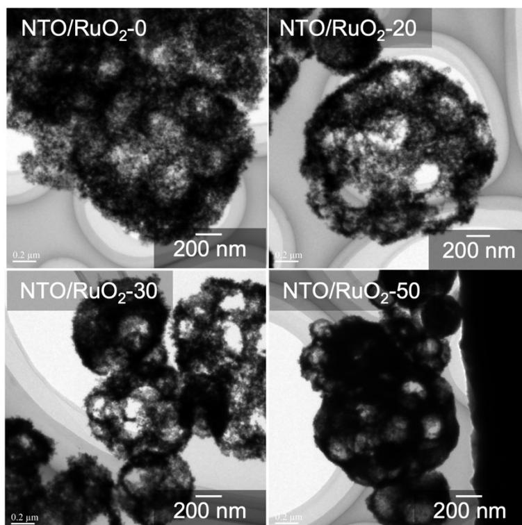
**Figure S2.** STEM images of macroporous NTO/ RuO<sub>2</sub> particles synthesized with different concentrations of RuO<sub>2</sub> binder.
