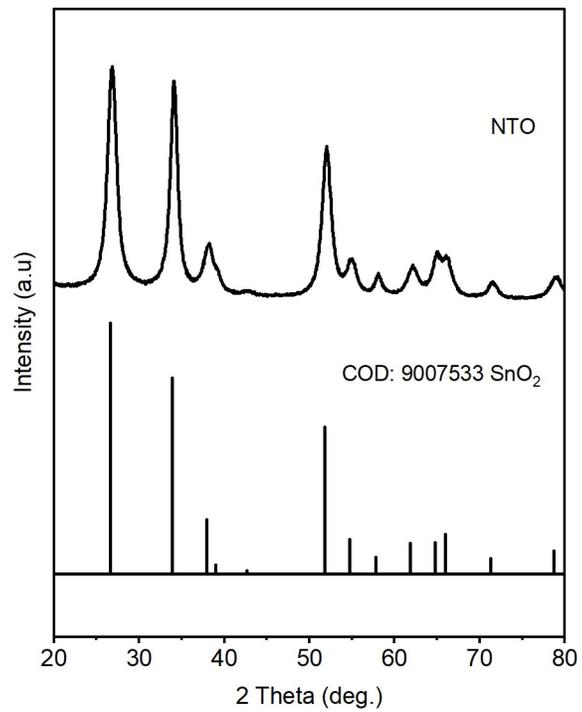
**Figure S5.** XRD patterns of NTO nanoparticles.
