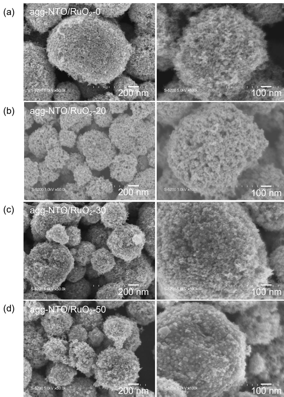
**Figure S4.** SEM images of aggregated NTO/RuO<sub>2</sub> particles with different RuO<sub>2</sub> binder contents: (a) agg-NTO/RuO<sub>2</sub>-0, (b) agg-NTO/RuO<sub>2</sub>-20, (c) agg-NTO/RuO<sub>2</sub>-30, and (d) agg-NTO/RuO<sub>2</sub>-50 particles.
