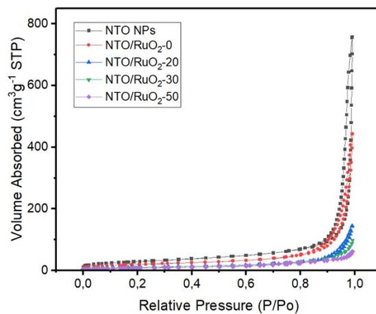
**Figure S3.** BET nitrogen adsorption isotherm plots of NTO nanoparticles and macroporous NTO/RuO<sub>2</sub> particles.
