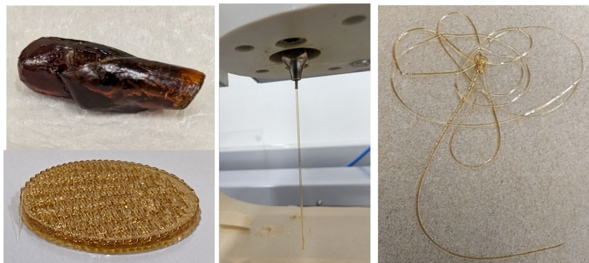
Extrusion of PET-DGA-im-C 6 -Tf 2 N ionene fibers
