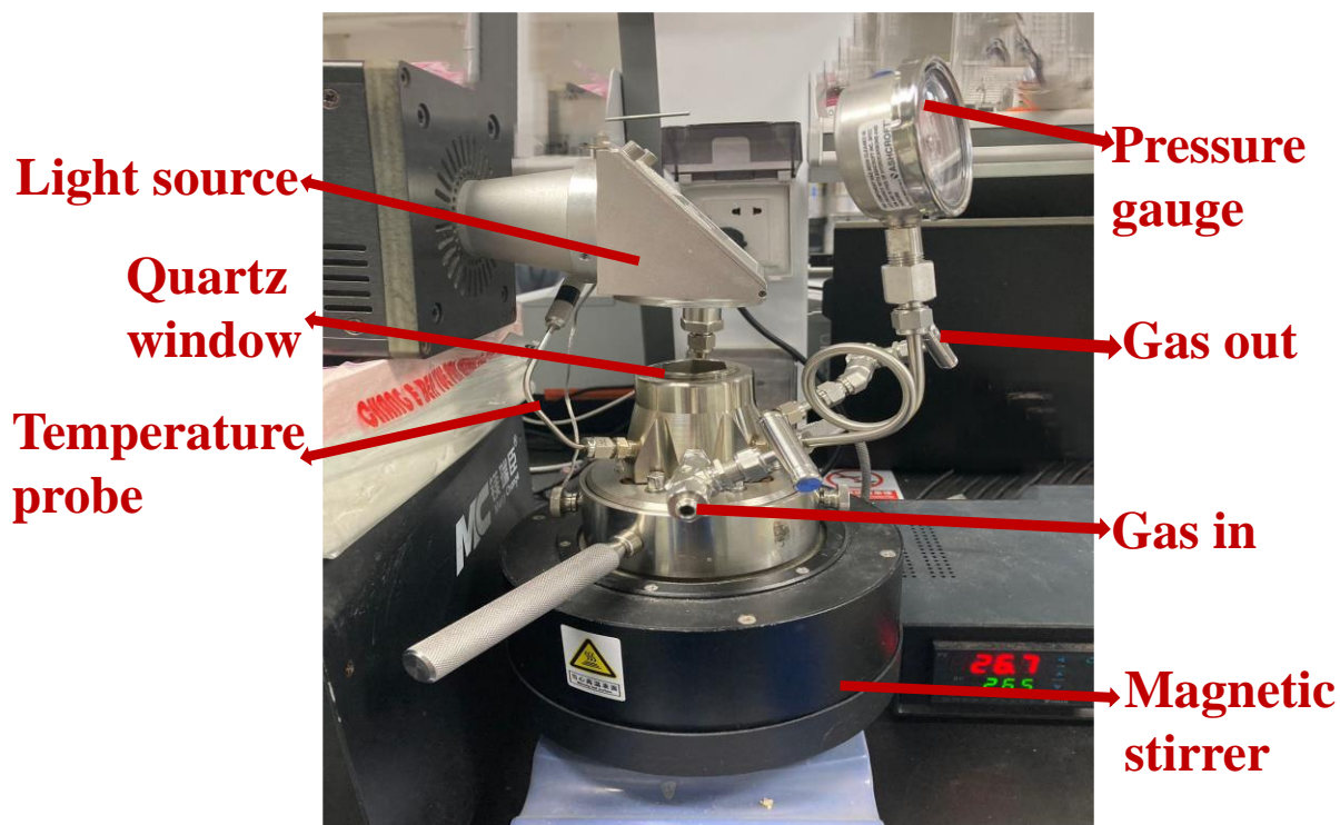
Fig. S1. Batch-type photoreactor experimental set-up
