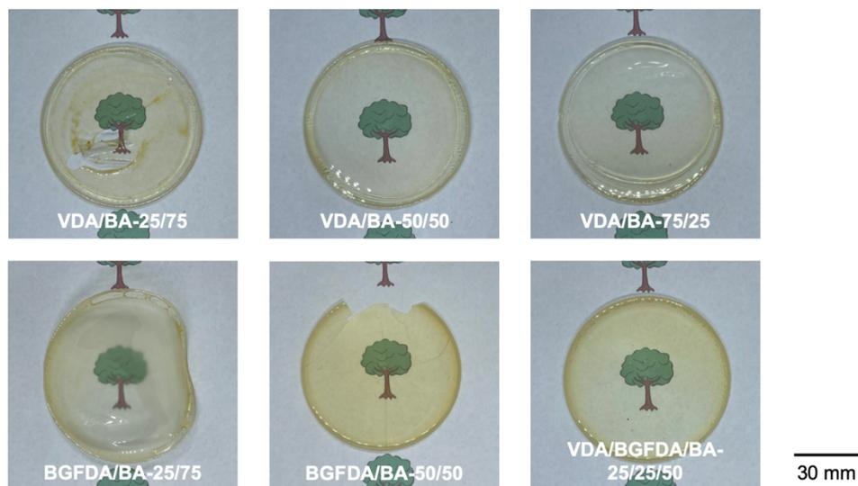
Fig. S6 Optical images of each acrylate networks after thermal post-curing with a film thickness  $\sim 0.2$  mm
