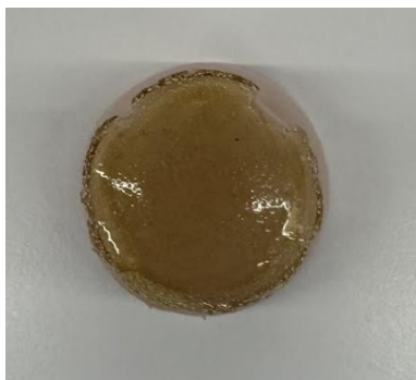
Figure S20. Image of Part A (vinyl-terminated PDMS) after inverse vulcanisation with 10 wt% sulfur at 180°C.
